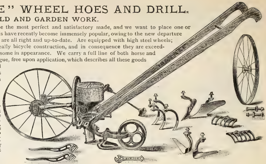
THE "IRON AGE" COMBINED SEED DRILL AND WHEEL HOE.
